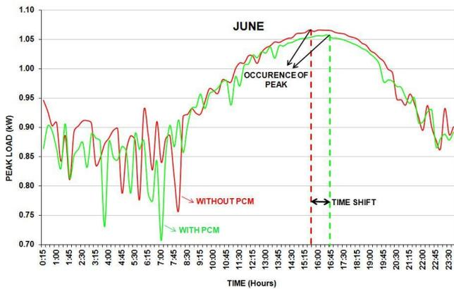
Figure 3: EXPERIMENTAL PEAK CURVE FOR JUNE
