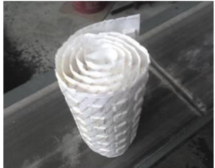
**Figure 1: BIOPCM MAT USED IN WALLS**
