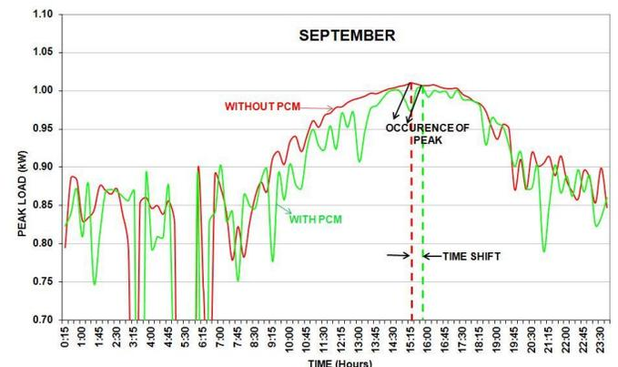
Figure 6: EXPERIMENTAL PEAK CURVE FOR SEPTEMBER
