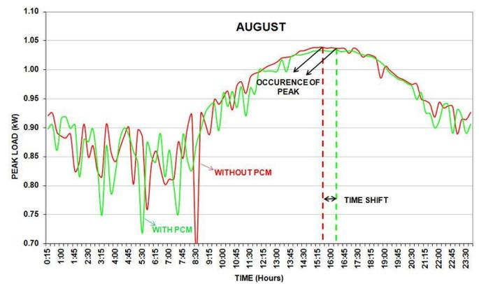
Figure 5: EXPERIMENTAL PEAK CURVE FOR AUGUST
